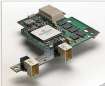
NE020BCH / KX4 Dual port CFFh form factor
